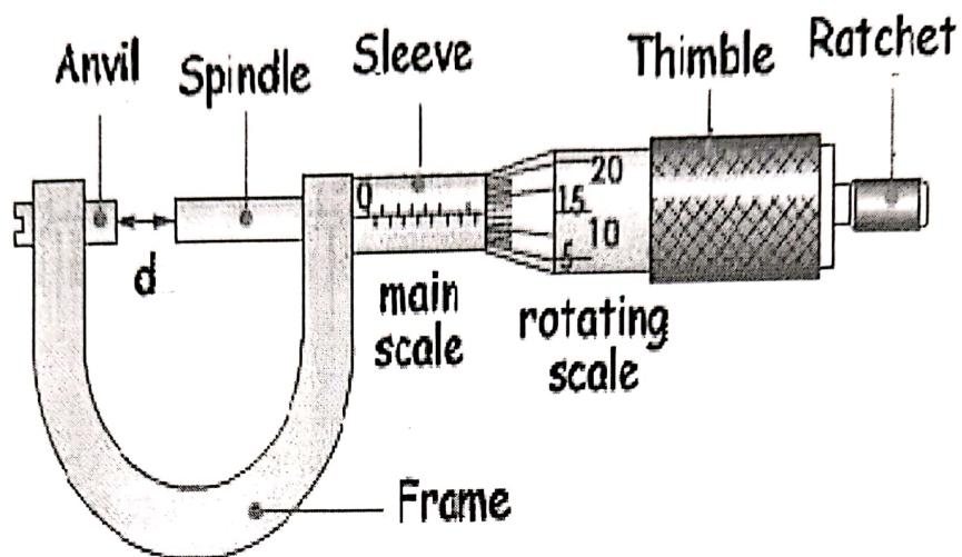
For example for a screw gauge with a pitch of 1mm and 100 divisions on the circular scale. The least count is =  $1 \text{ mm}/100 = 0.01 \text{ mm}$
